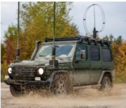
Figure 14 - Vehicle mounted loop antenna
