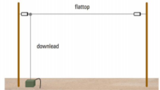
Figure 13 - Unbalanced wire (inverted L)
