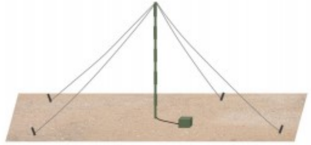
Figure 12 - Inverted Vee (turnstile configuration)
