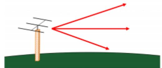
Figure 2 - Line of sight propagation
