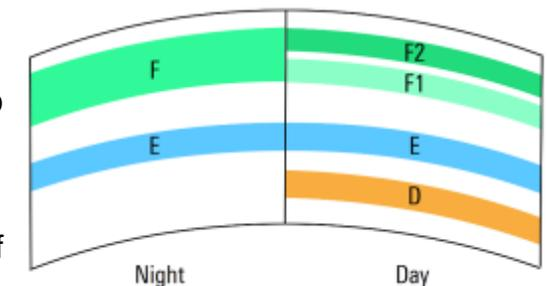
Figure 5 - Ionospheric layers
