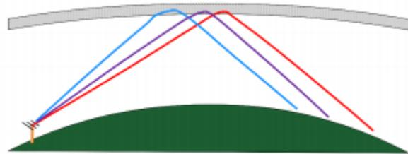
Figure 4 - Skywave propagation
