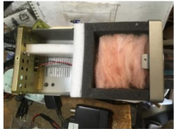
Added soft insulation to dampen the sound back wave.
