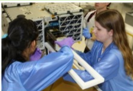
Students insert the Bevo-2 CubeSat into the AggieSat4 package. [Texas A&M photo by Dexter Becklund]
