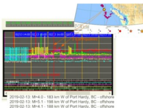
The RF Seismograph indicates an increase in 80-meter noise (red trace) corresponding with an earthquake west of Port Hardy, British Columbia.
