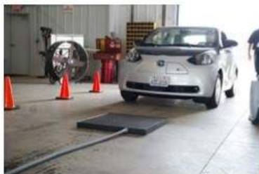
Researchers at Oak Ridge National Laboratory test a wireless power transfer charger on a fully electric vehicle. [US Department of Energy photo]
