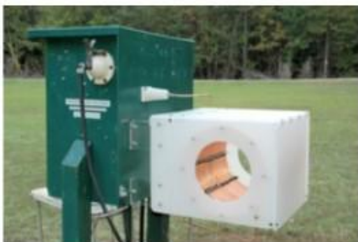
Ralph Hartwell, W5JGV, in Louisiana, takes part in the WD2XSH experiment. This is the base loading coil and antenna tuning unit for his 600 meter vertical.
