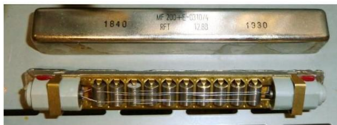
Figure 2: A Mechanical Filter
